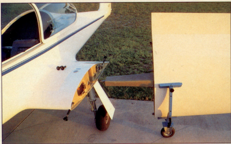
Taifun's wing demates outboard of landing gear and fuel cells. Push rods and roller bearings connect controls from fuselage automatically.
