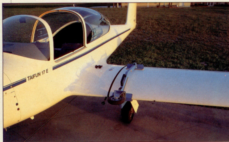
Taifun's wing demates outboard of landing gear and fuel cells. Push rods and roller bearings connect controls from fuselage automatically.
